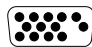
HD15 Male—VGA (Pins 9 and 15 are removed on the EVNPS05 and EVNPS07 for compatibility with all VGA computers. EVNPS10 supports all 15 pins.)
