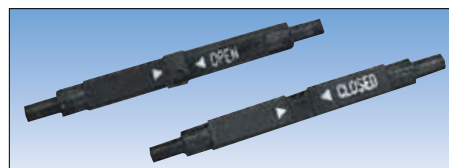
You won't have gluing or alignment problems with the No-Adhesive Mechanical Splice (FO030). A cam locks the fibers into position for accurate alignment.
