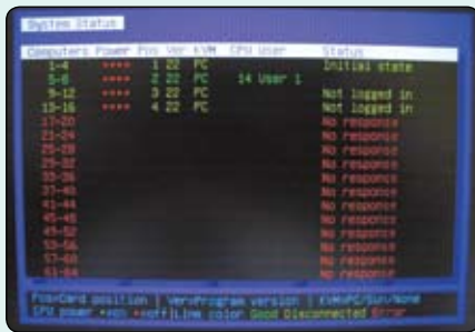
On-screen menus make it easy to identify the system status of computers in an installation.
