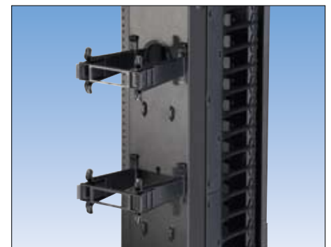
The Vertical Post & Gate Kit has 10 sets of posts and gates that snap together quickly. Each set consists of two posts and one gate. The posts snap into prepunched holes on the cable manager. The gates swivel 280° in either direction to allow easy cable access.
